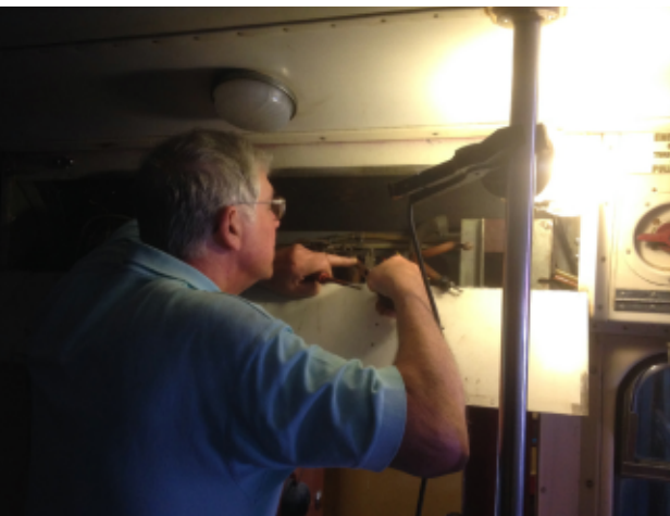
Bruce Lake adjusting the switches in the rear door interlock mechanism
